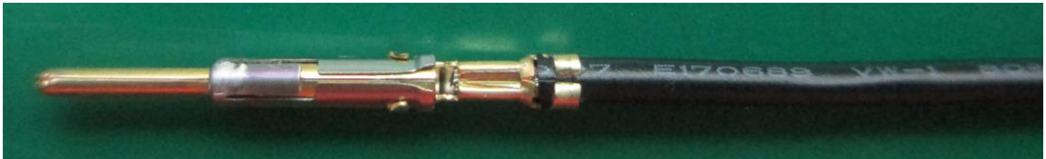
铆压完成后图示 Picture after finishing the crimping
