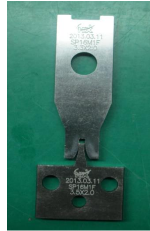
铆压完成后图示 Picture after finishing the crimping
